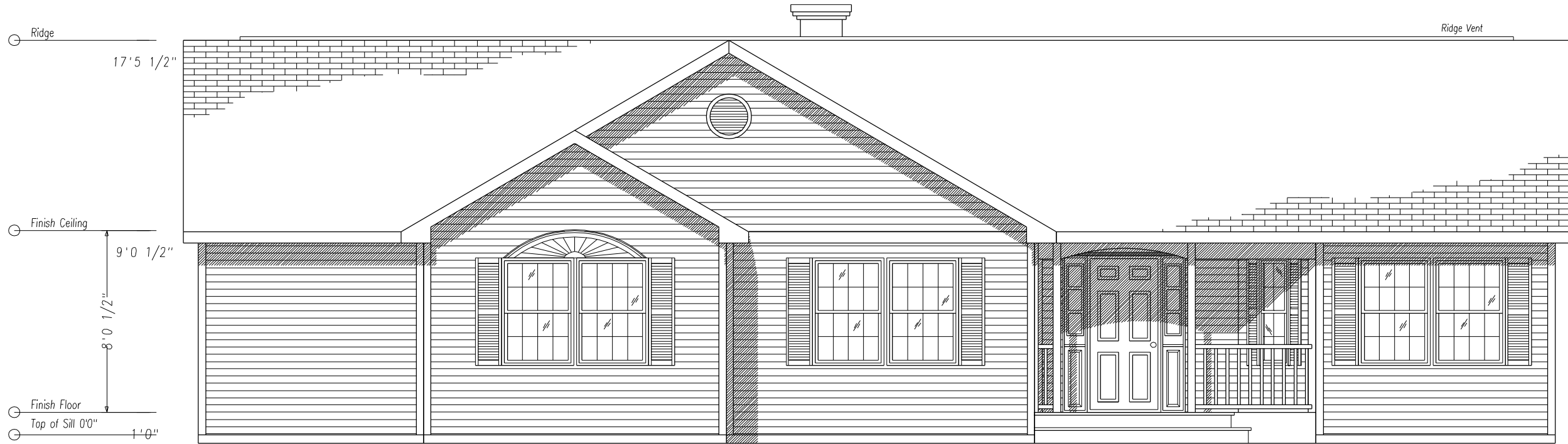
Front Elevation Scale: 3/16" = 1'0"
