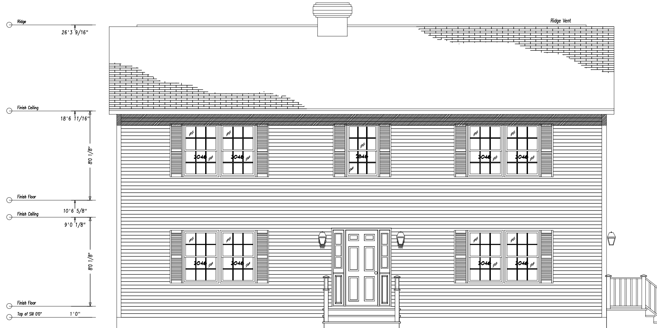
Front Elevation Scale: 3/16" = 1' 0"
