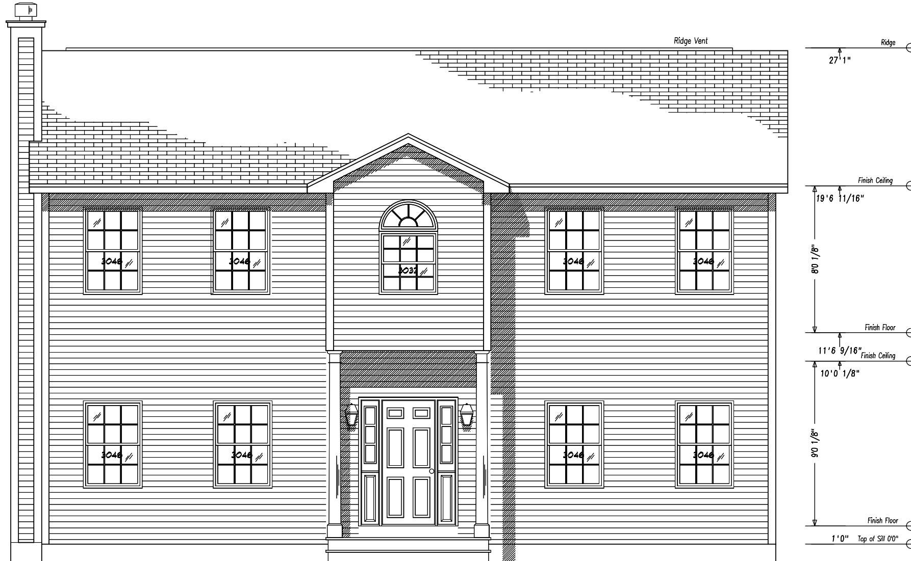
Front Elevation Scale: 3/16" = 1'0"
